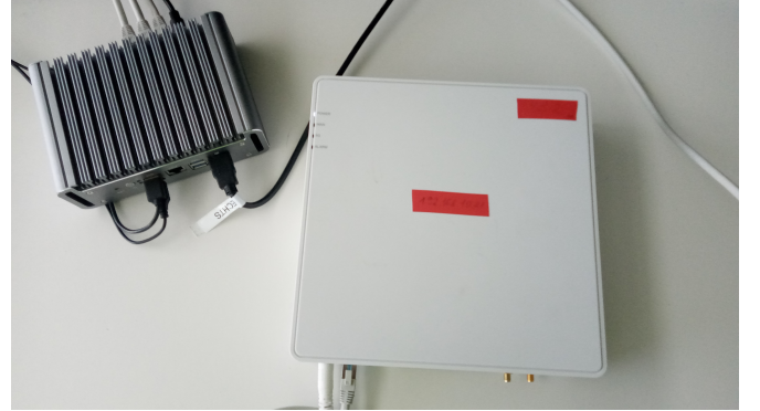
Fig. 9. Minimal nomadic 5G system.
