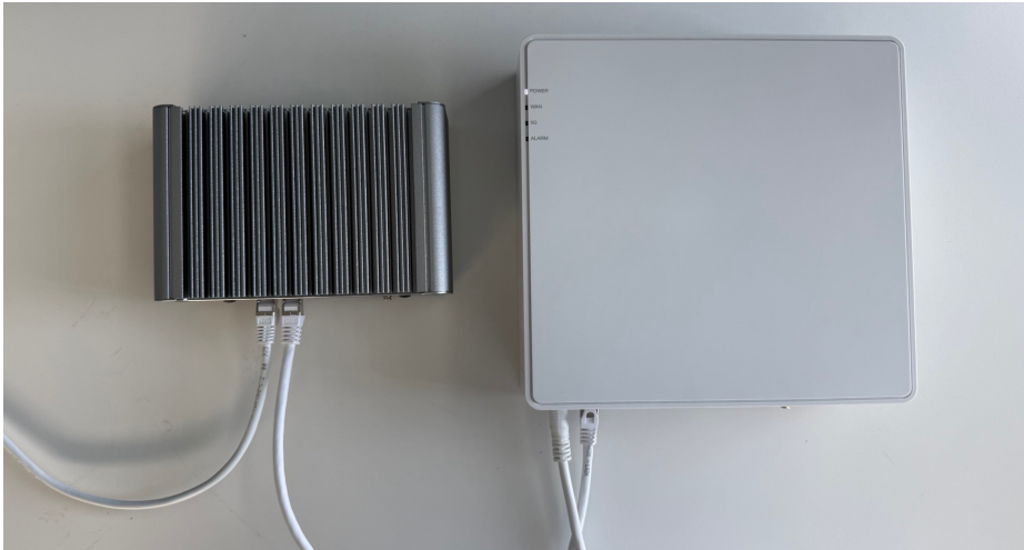
Minimal system: fanless PC + Sercomm gNB
